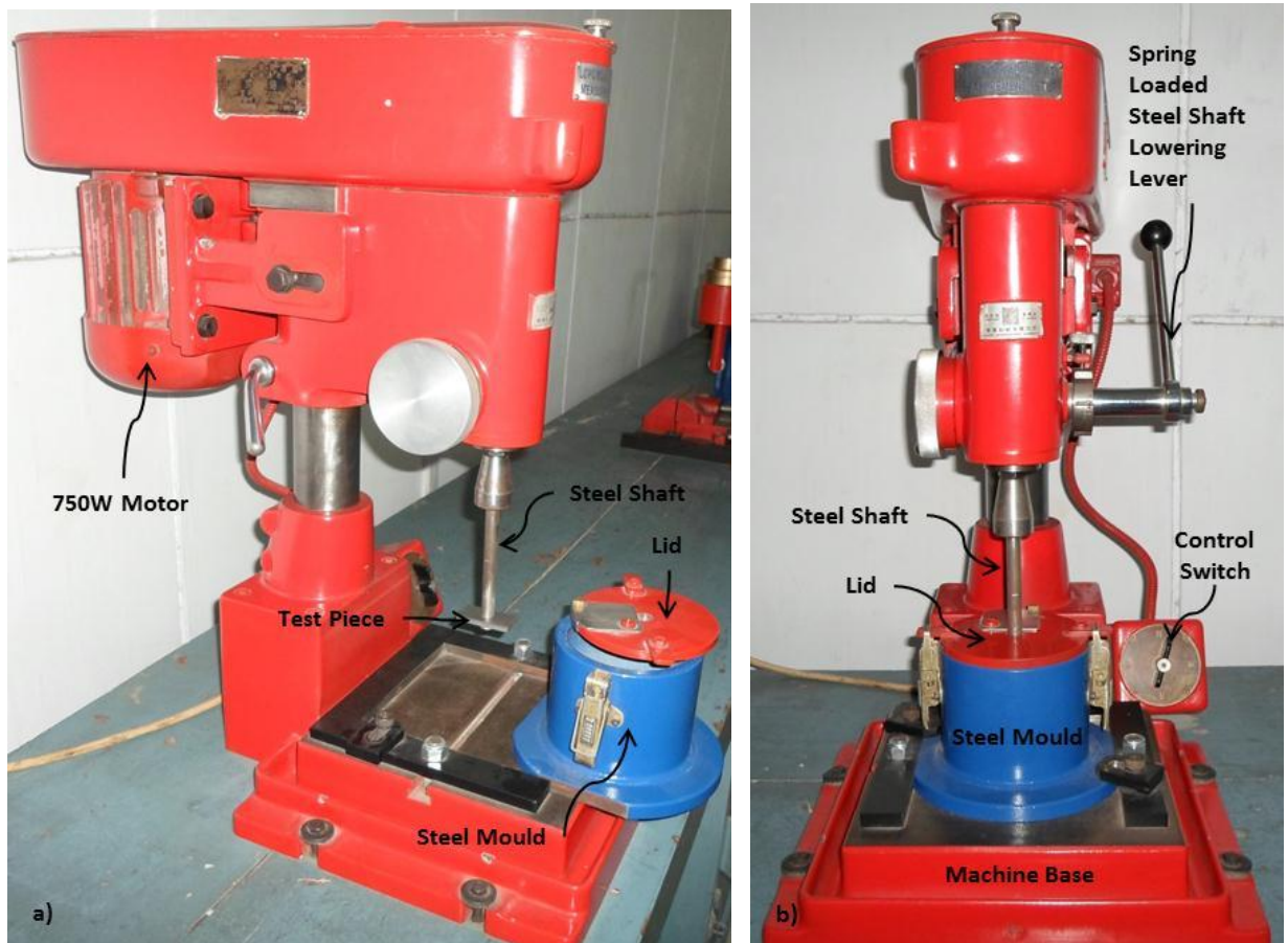
Figure 3.5. The LCPC rock abrasivity measurement apparatus (a) side view (b) front view.
