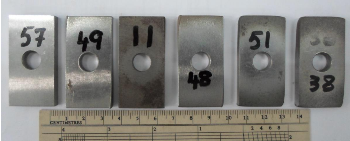
Figure 3.8. LCPC inserts before and after test performance. 57- new test piece, 49- tested on Limestone-3 (ABR= 8 g/t), 11- tested on Sandstone-2 (ABR= 62 g/t), 48- tested on Dolomite-3 (ABR= 336 g/t), 51- tested on Quartzite-1(ABR= 498.50 g/t), 38- tested on Sandstone-16 (ABR= 1444.56 g/t).
