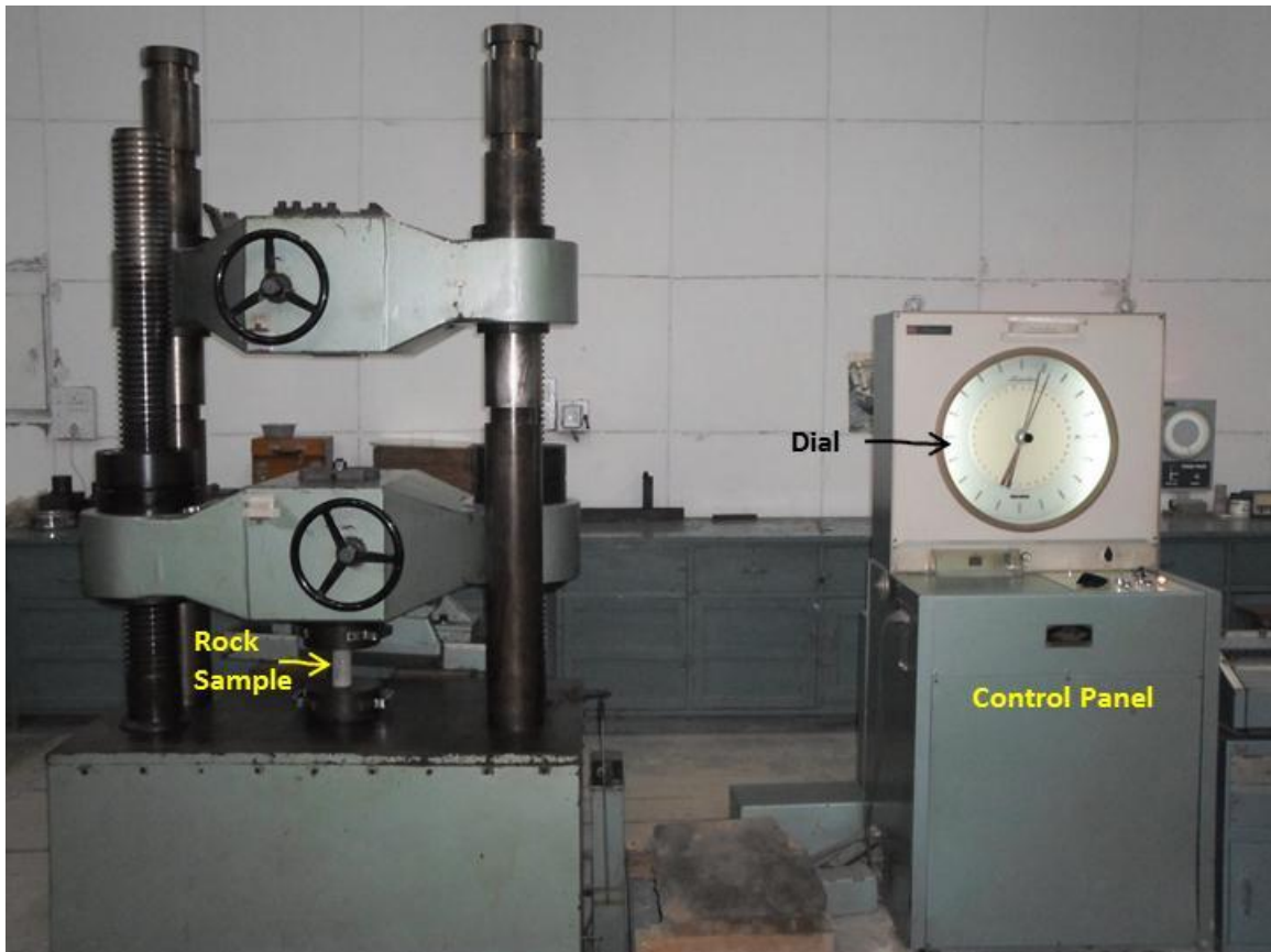
Figure 3.18. A view of Shimadzu 200 tons universal testing machine used for performing mechanical rock properties tests.
