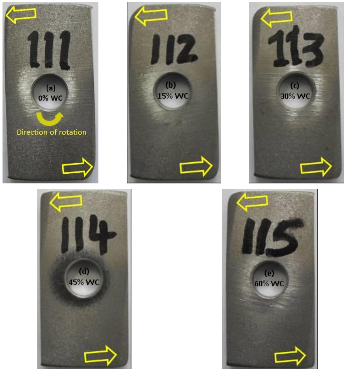
Figure 7.4. LCPC inserts tested on Andesite rock sample (a) in dry state (b) at 15% water content (c) at 30% water content (d) at 45% water content (e) at 60% water content.
