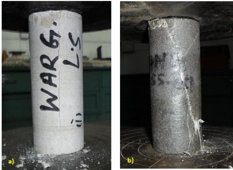
Figure 3.19. View of rock cores after performing UCS tests (a) Limestone-4 rock core tested in the dry state (b) a fully saturated core of Sandstone-18 rock sample after failure.
