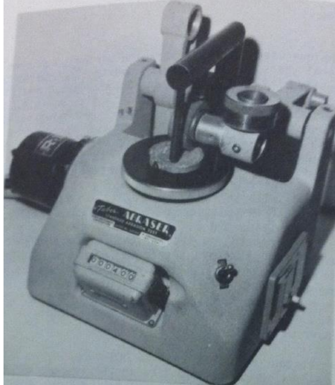
Figure 2.20. Modified Taber abrasion test (after Tarkoy, 1973).
