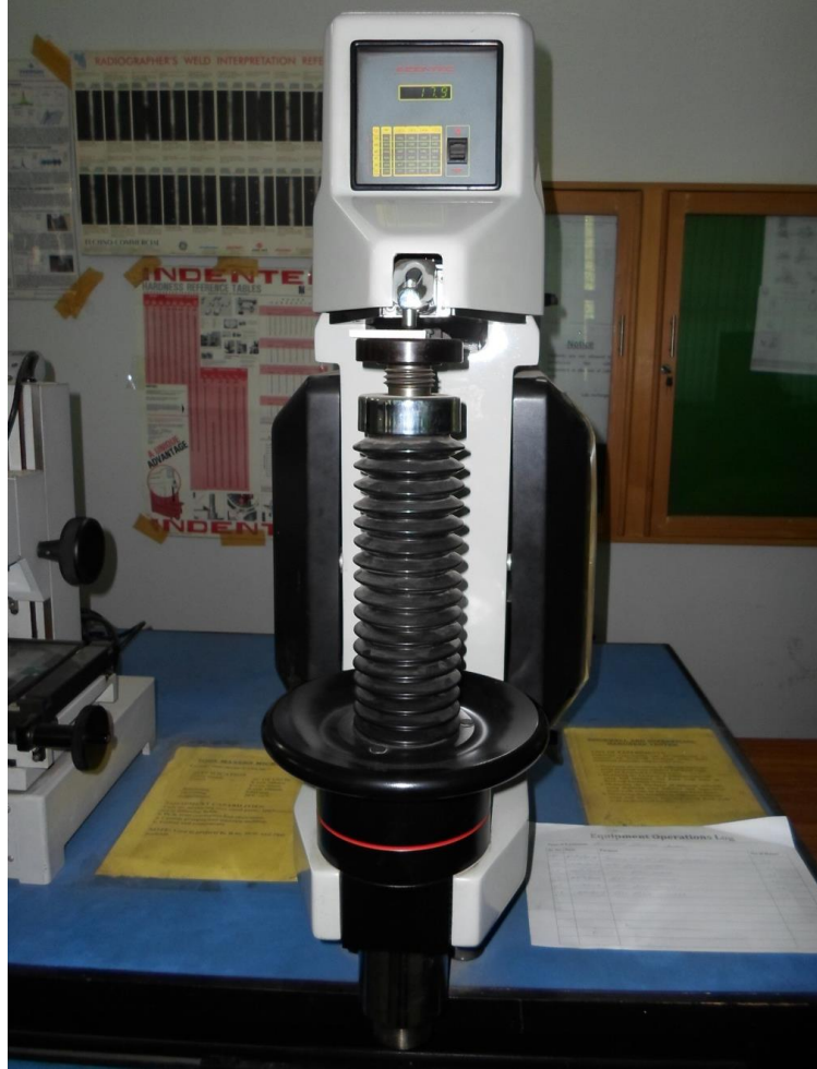
Figure 3.6. A view of Rockwell hardness testing machine captured while testing hardness of a LCPC test insert.
