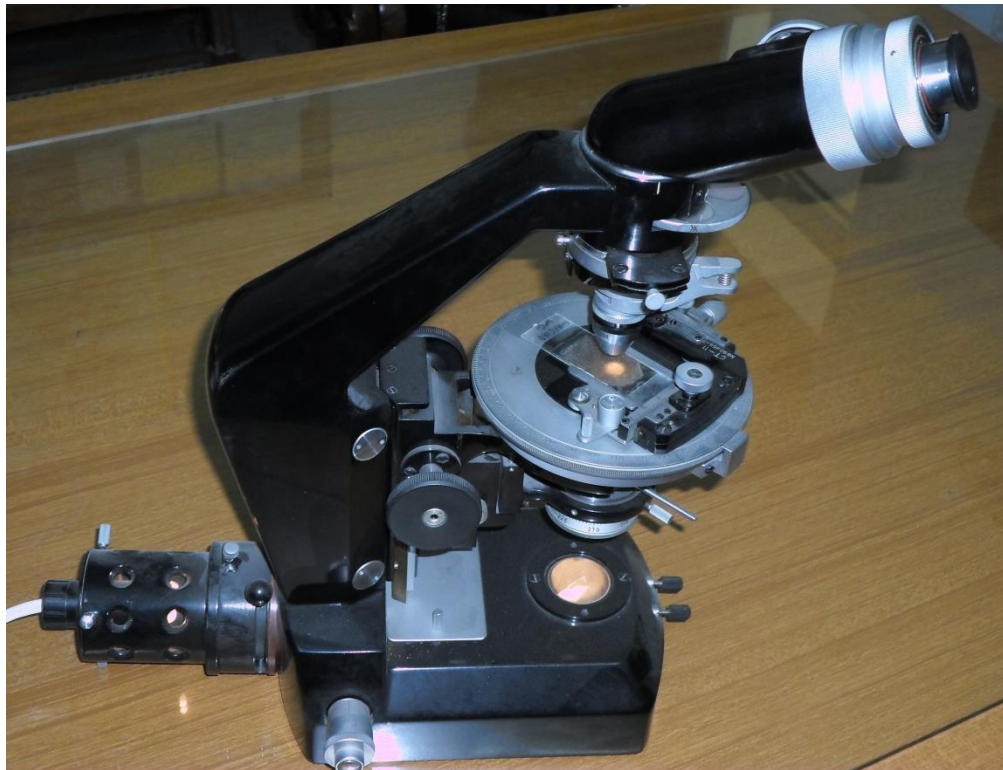
Figure 3.15. MNH-8 Russian, polarized light microscope used in the petrographic study.
