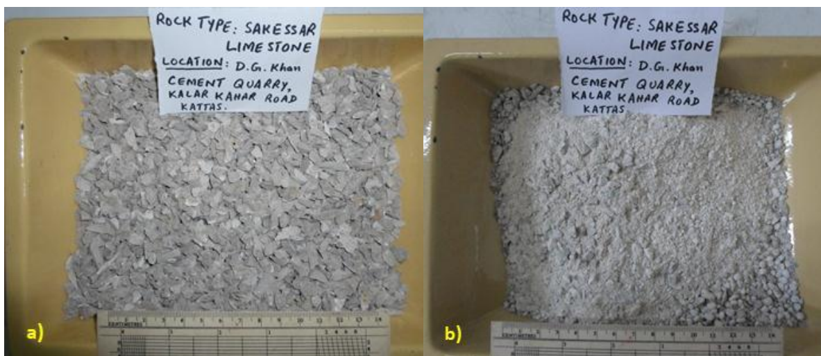
Figure 3.7. (a) A view of prepared rock fraction before LCPC test (b) a view of rock fraction after LCPC test, where the rock breakability effect can be noticed.
