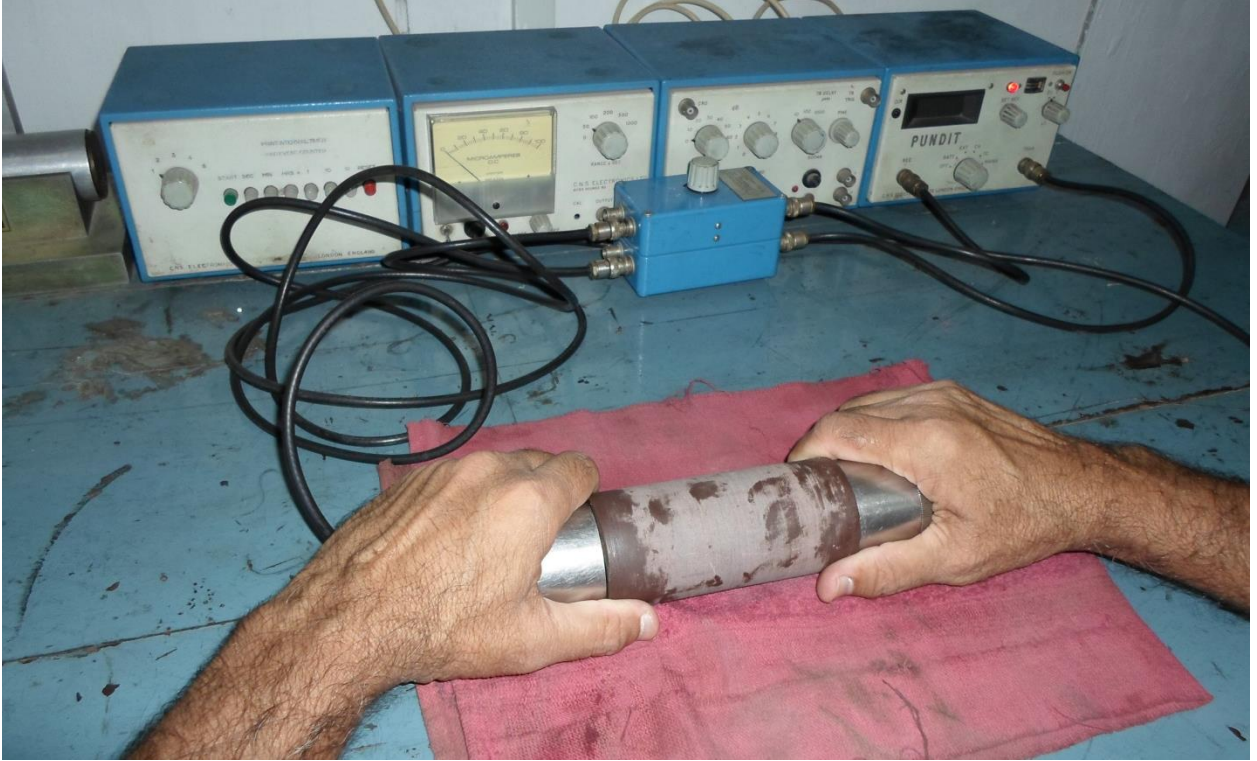
Figure 3.21. View of measuring P-wave velocity of a Sandstone -16 rock sample using PUNDIT.
