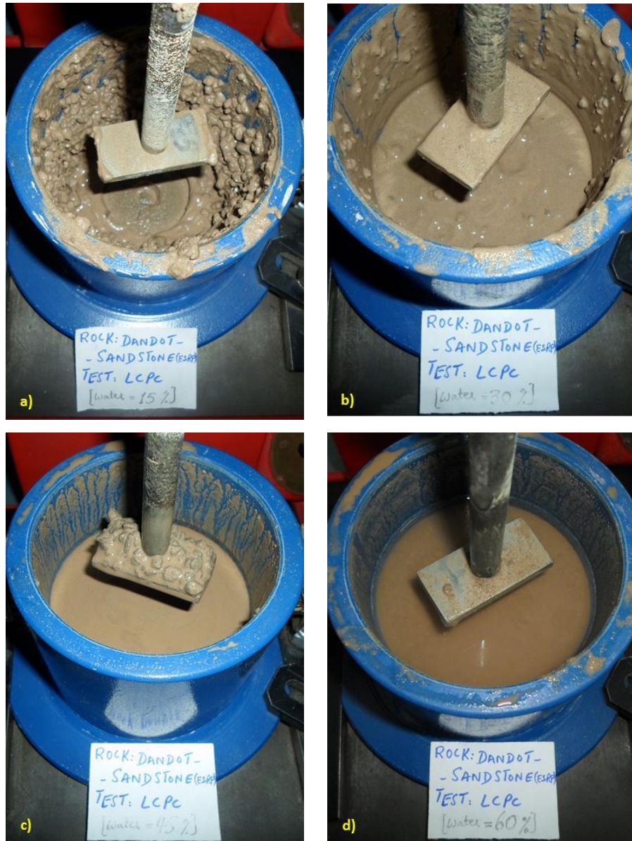
Figure 3.9. LCPC saturated tests performed on Sandstone-5 rock sample (a) at 15% water content; (b) at 30% water content; (c) at 45% water content; (d) at 60% water content.
