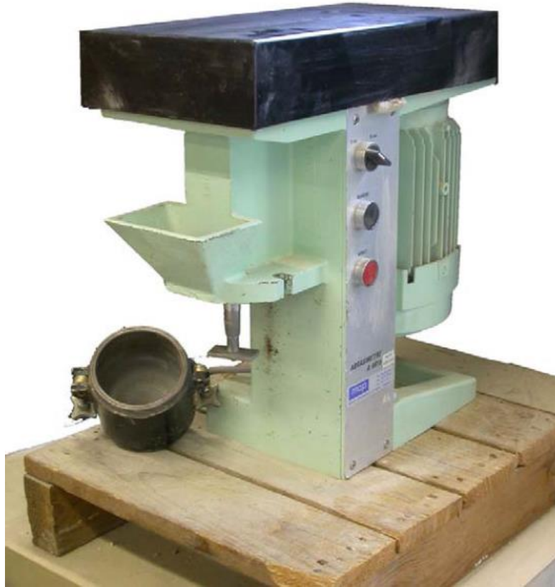
Figure 2.13. LCPC rock abrasivity testing device (after Nilsen et al., 2007).
