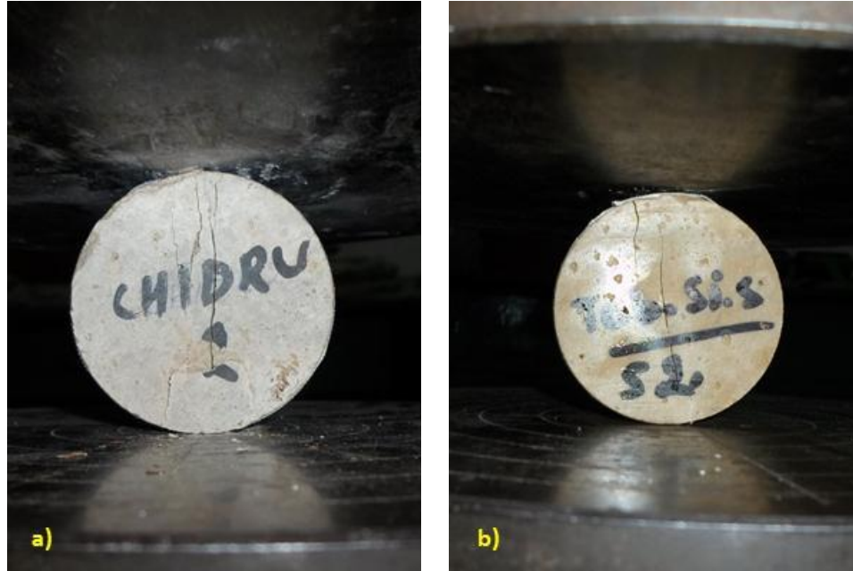
Figure 3.20. View of rock disc after performing BTS tests (a) a failed disc of Sandstone-7 rock sample tested in the dry condition (b) a fully saturated disc of Siltstone-2 rock sample after failure.
