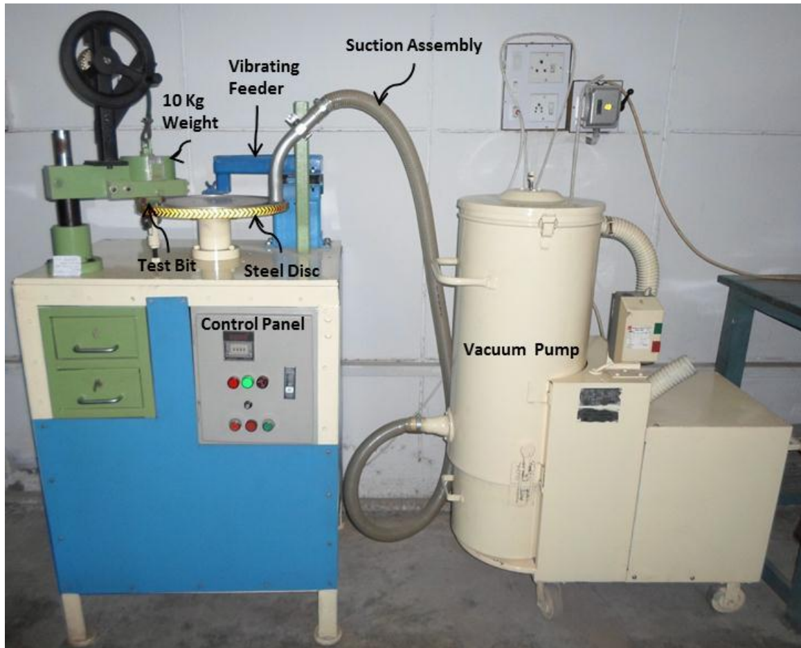
Figure 3.12. NTNU/SINTEF Abrasion Value Steel Cutters (AVS) test apparatus
