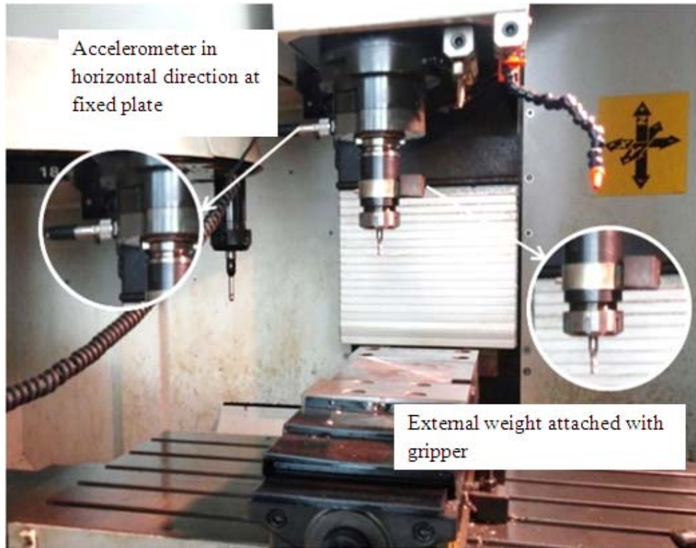
Figure 4.10: Experimental setup for inducing forced vibrations
