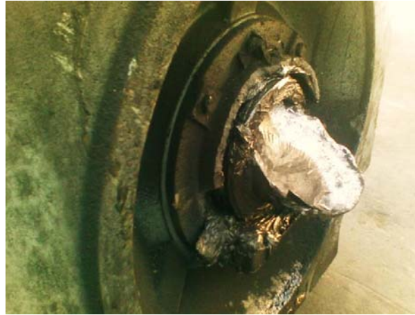
c) Motor shaft failure due to vibration [12]
