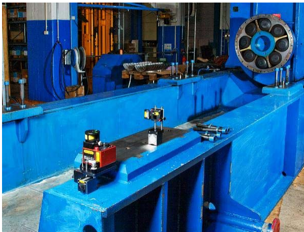
c) Flatness check for machine bed
