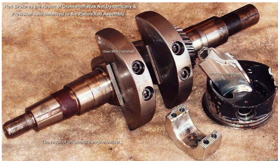
b) Breakage of rod due to vibrations caused by crankshaft looseness [12]
