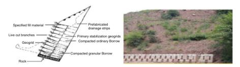
Fig. 8.5 Block retaining wall
