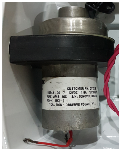
Figure 2.12 Vacuum pump for insulation
