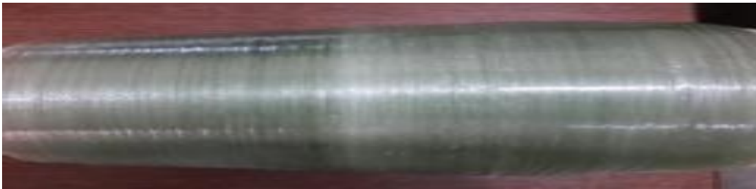
Figure 11 Picture of Cured Pipe at 140°C at Production Unit
