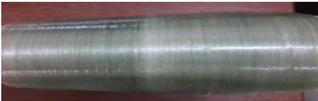
Figure 12 Picture of Cured Pipe at 130°C at Production Unit
