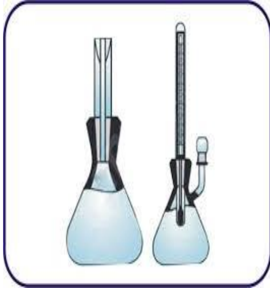
Figure 5 Instrument for determine specific gravity
