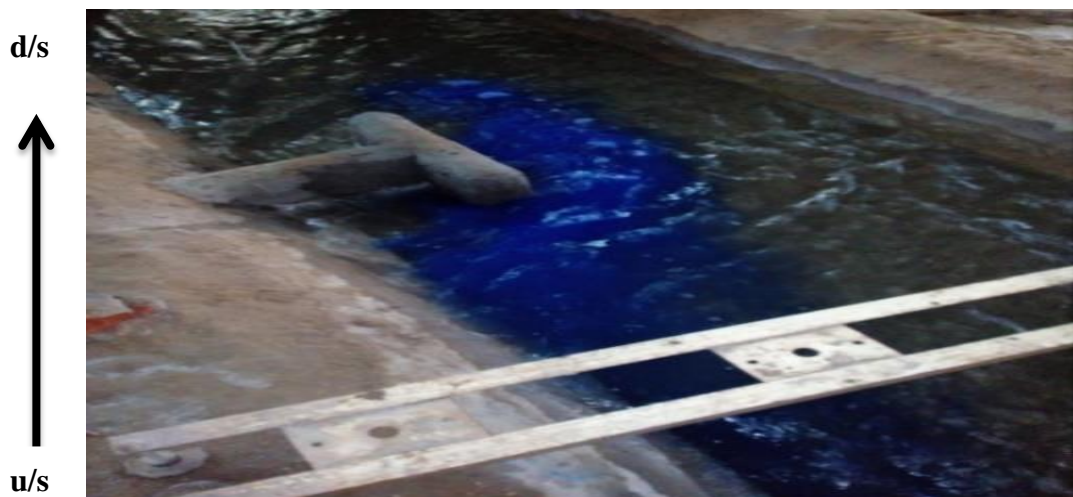
Figure 4.84: Direction of velocity currents in T-Spur at 0.30 cusec/m
