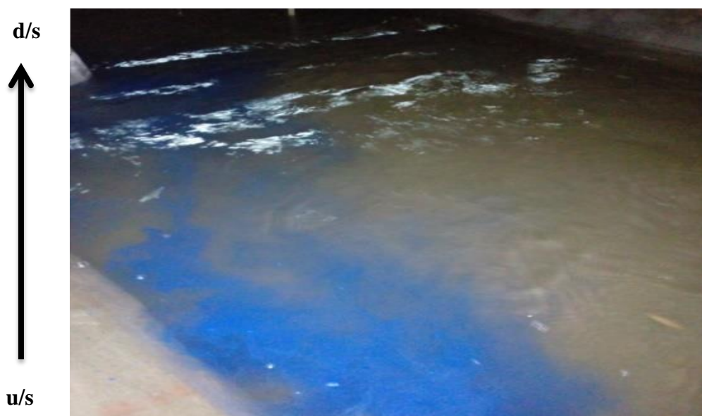
Figure 4.7: Direction of velocity currents at 0.20 cusec/m
