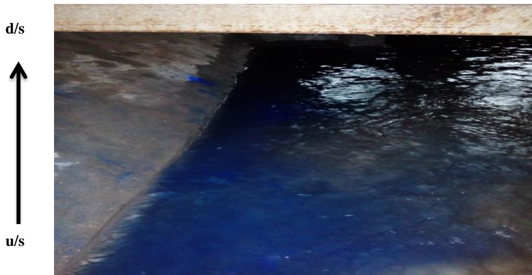
Figure 4.76: Direction of velocity currents in T-spur at 0.15 cusec/m
