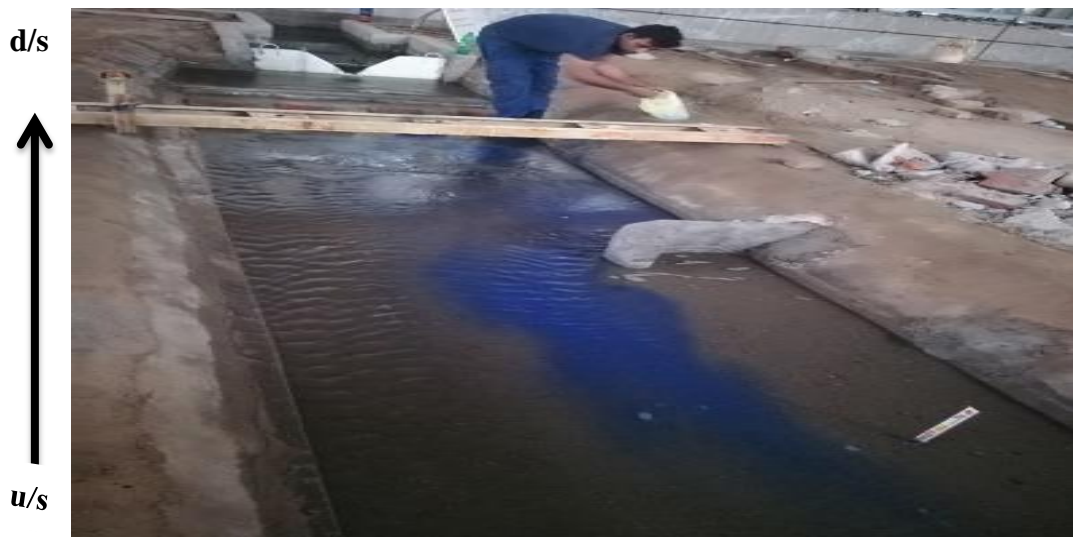
Figure 4.108: Direction of Deflection currents in hockey spur at 0.20 cusec/m
