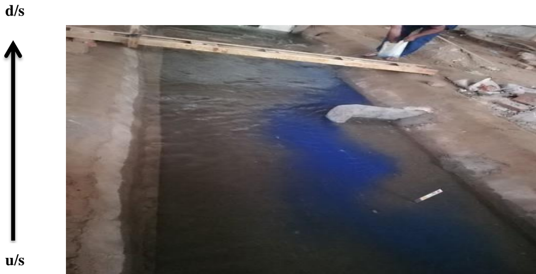
Figure 4.112: Direction of water currents in hockey spur at 0.30 cusec/m
