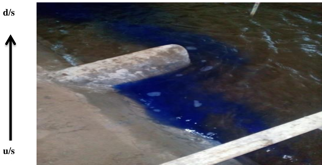
Figure 4.11: Direction of velocity currents at 0.30 cusec/m
