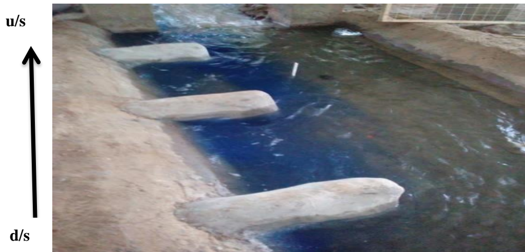
Figure 4.53: Direction of velocity currents in three spur at 0.30 cusec/m
