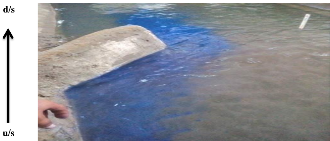
Figure 4.35: Direction of velocity currents of attracting spur at 0.20 cusec/m discharge
