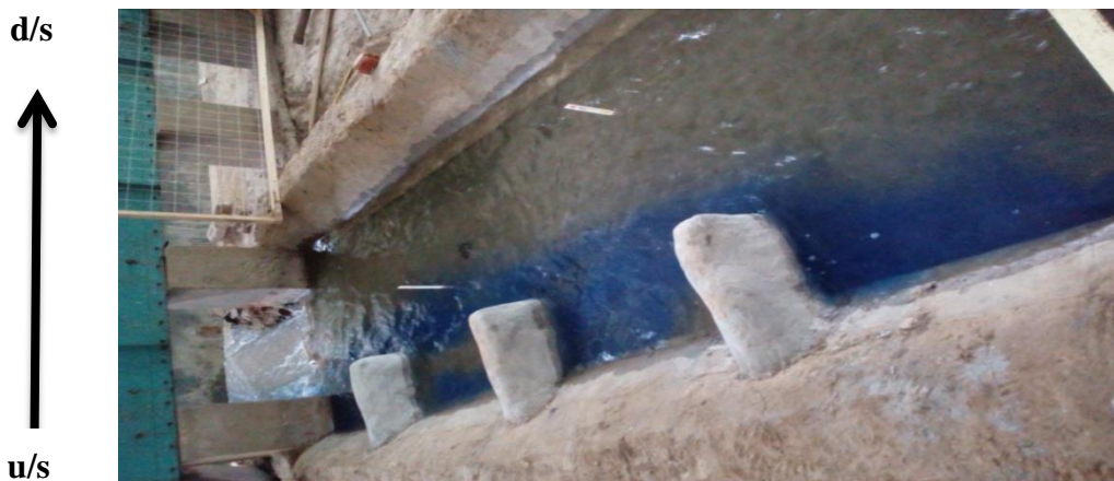
Figure 4.49: Direction of velocity currents in three spur at 0.20 cusec/m
