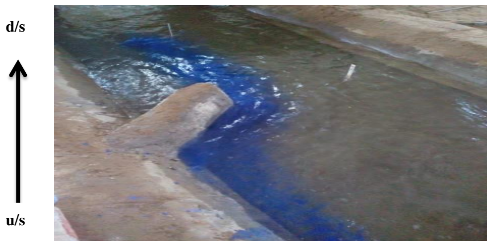
Figure 4.39: Direction of velocity currents of attracting spur at 0.30 cusec/m discharge
