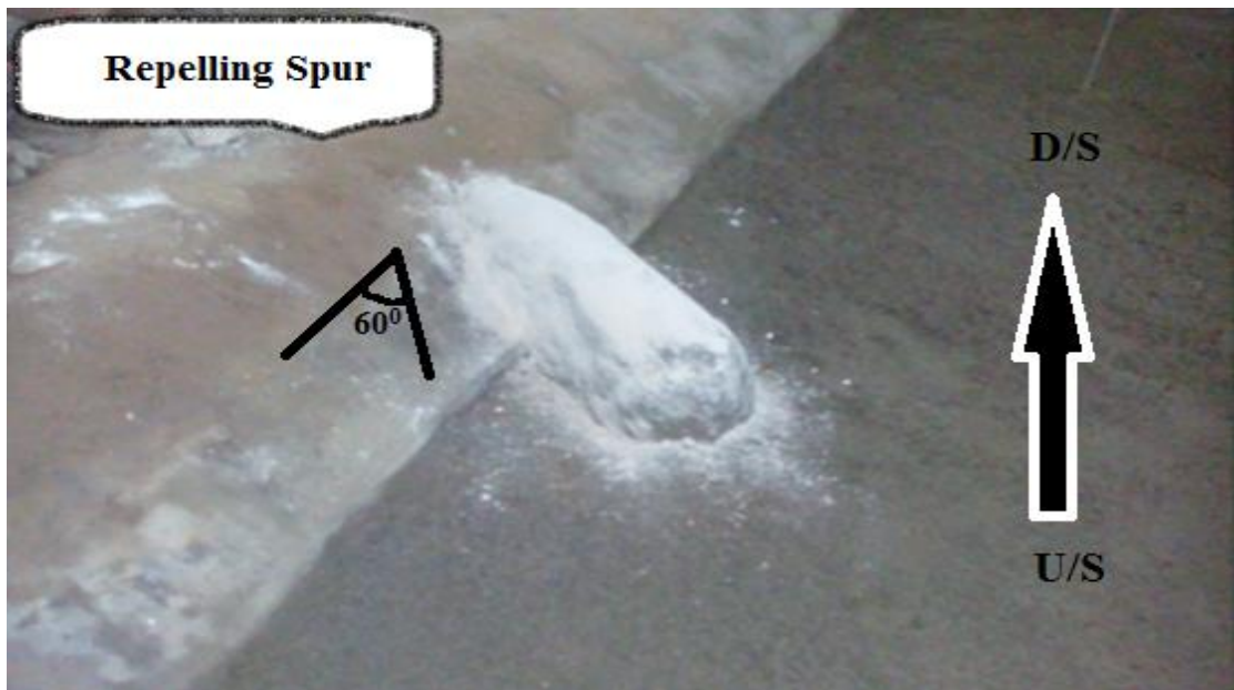
Figure 3.5: Spur type: repelling spur (Angle 60)
