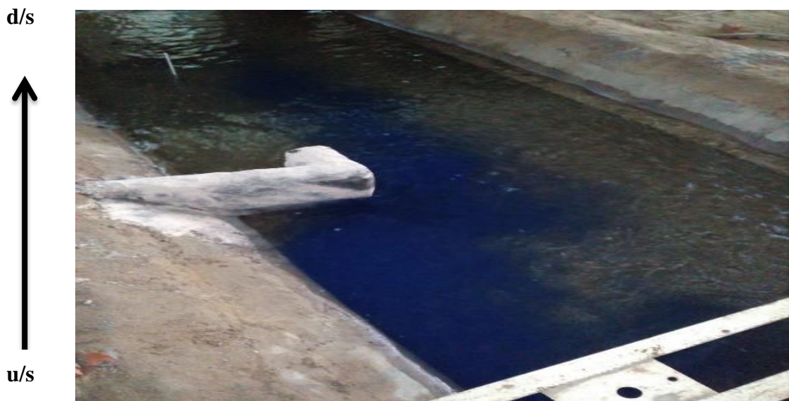
Figure 4.90: Direction of currents velocity J-Spur at 0.15 cusec/m
