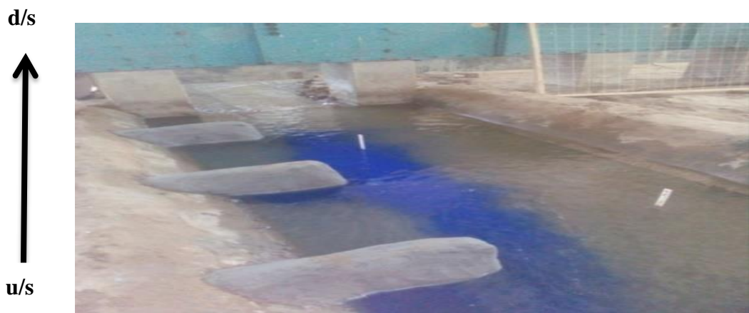
Figure 4.45: Direction of velocity currents in three spurs at 0.15 cusec/m
