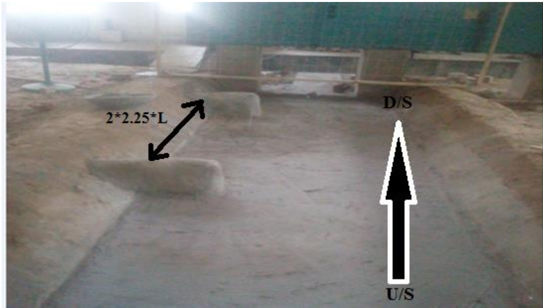
Figure 3.8: Series of two spur spacing
