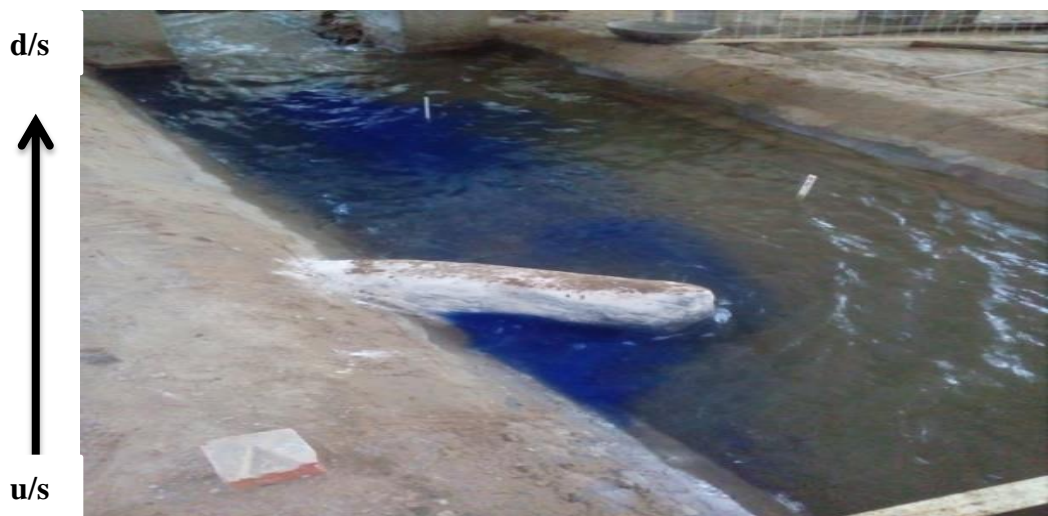
Figure 4.25: Direction of velocity currents of repelling spur at 0.30 cusec/m
