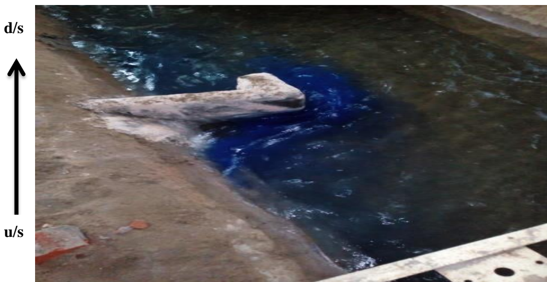
Figure 4.104: Direction of Deflection currents in hockey spur at 0.15 cusec/m.
