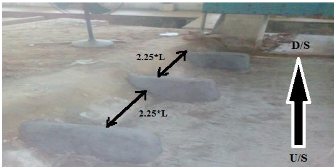
Figure 3.7: Series of three Spur spacing
