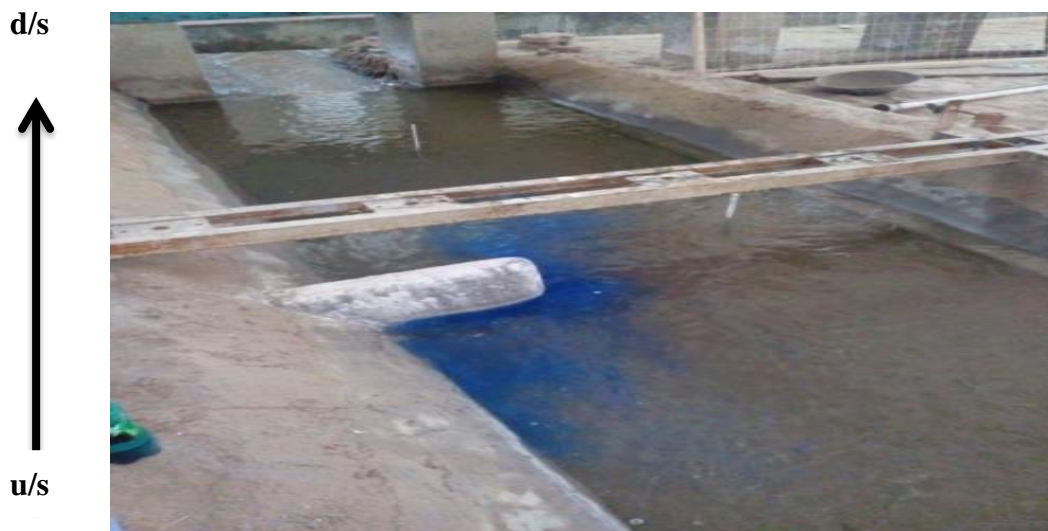
Figure 4.3: Direction of velocity currents at 0.15 cusec/m
