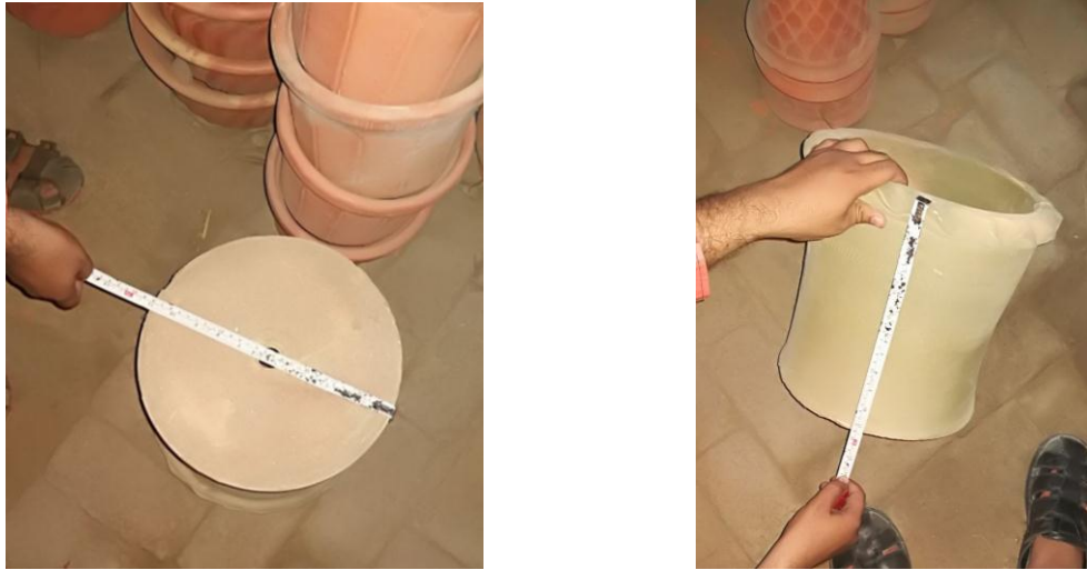
Fig-2. 5 10 inch Dia. and 10 inch height of cylindrical shape burnt clay Pots
