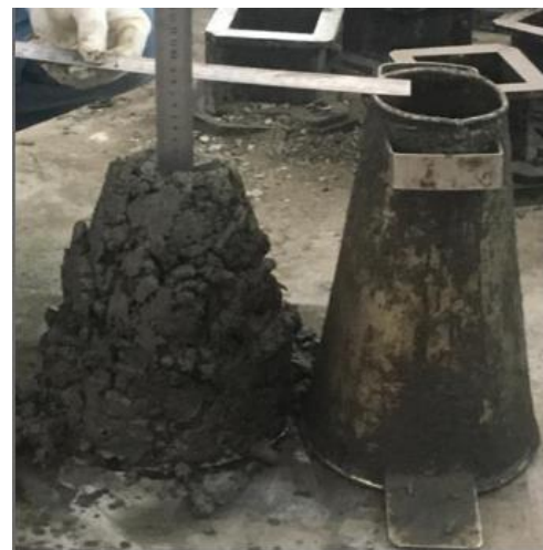
(b) Slump value of concrete
