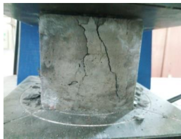
(b) Specimen at first crack
