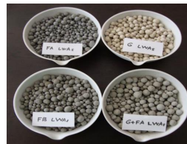
Fly ash and Slag Aggregates [7]
