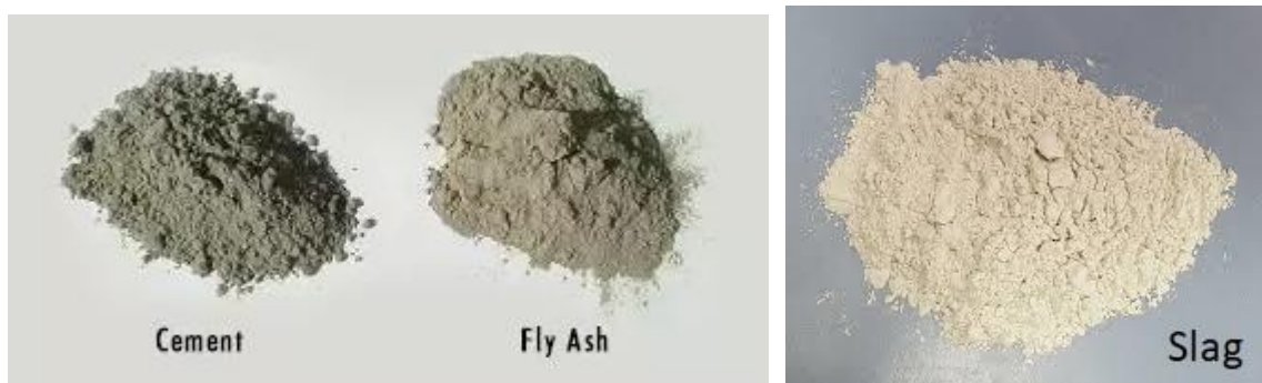
Figure 2. Different binder or precursor used in this work
