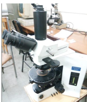
(a) Petrographic microscope
