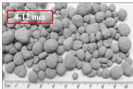
Sewage sludge ash aggregates [39]
