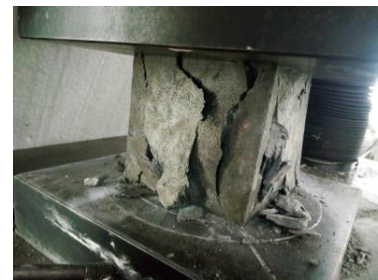
(c) Fully cracked specimen
