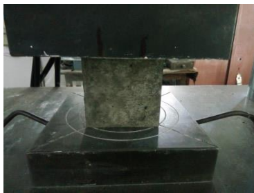
(a) Cube sample placed in UTM
