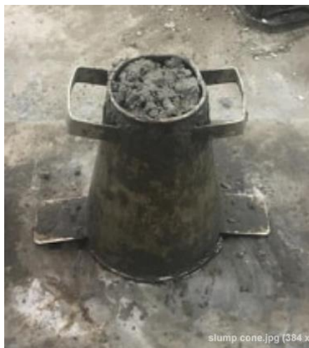
(a) Concrete filled slump cone
