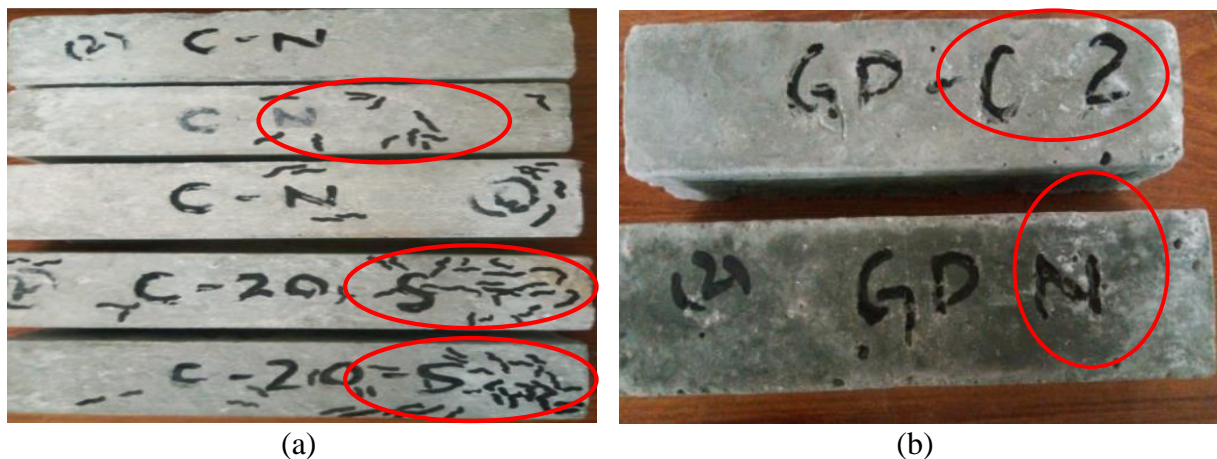
Figure 16. NaOH exposed specimens: (a) C-specimens exhibiting cracks, (b) G-specimens displaying leaching
