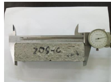
(c) Length change measurements
