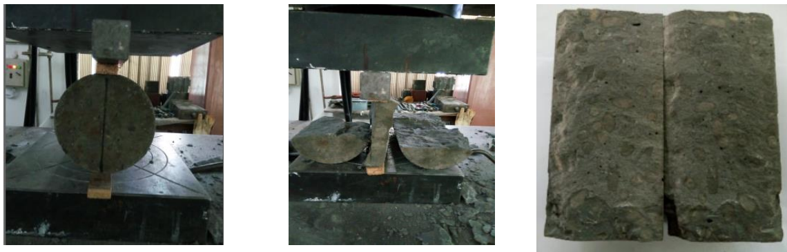
(a) Specimens placed in UTM (b) Specimen at failure (c) Specimen after failure
