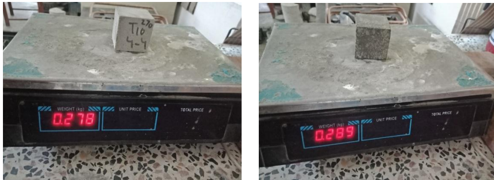
Figure 3.16: Dry and wet weight of mortar sample for water absorption test
