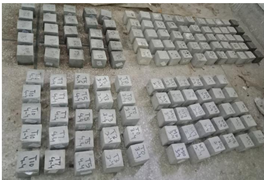
Figure 3.14: Prepared mortar samples for testing
