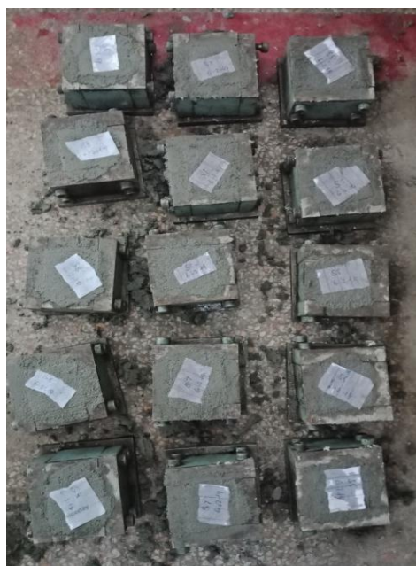
(f) Prepared mix in molds
