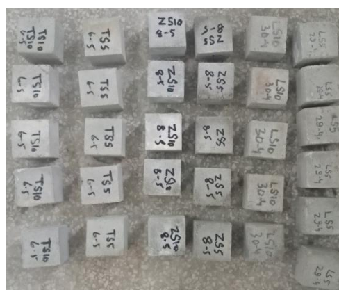
(h) Prepared samples of SBR latex modified with nano particles and Zinc Stearate
