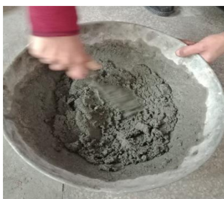
(e) Prepared mix of SBR powder modified mortar mix in molds
