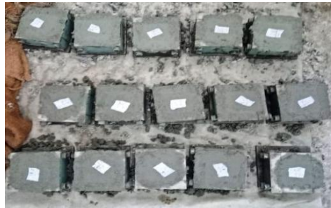
Figure 3.12: Prepared mortar mix filled in molds
