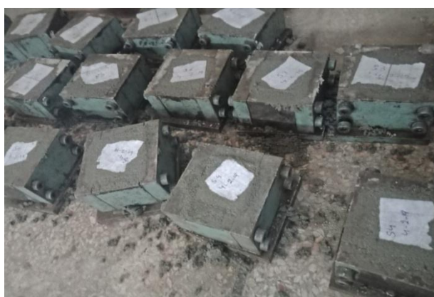
(g) Prepared mix in molds
