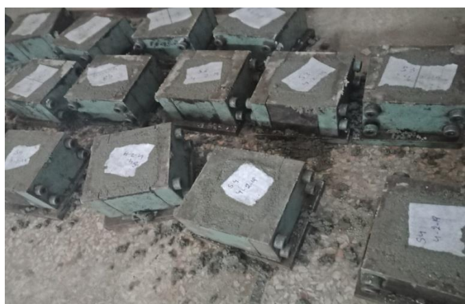
(f) Prepared mix in molds
