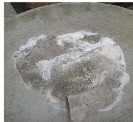
(b) Dry mixing of SBR powder and cement
