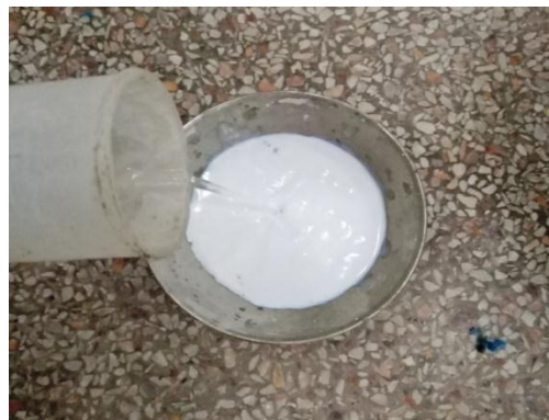
(b) Addition of SBR latex in water
