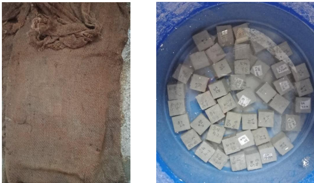
Figure 3.13: Wet curing and submerge curing of mortar cubes
