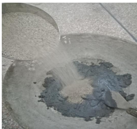
(e) Sand added into the mixture
