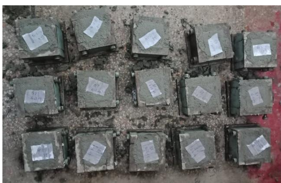
(g) Mortar mix poured in molds
