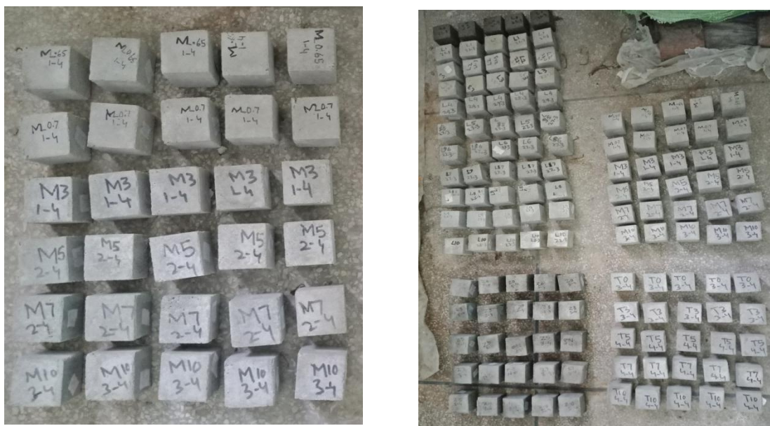
(h) Prepared samples of SBR powder modified with nano-particles and zinc stearate
